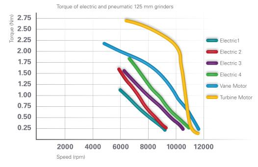
The power curves show the linear characteristics of the electric motor, the output increases continually as the motor gets more load. This would continue further, giving more power until the motor breaks. The same applies on the torque curves. To avoid damage to the motors, the test was stopped as the tool got
