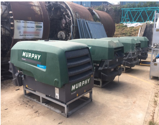
The frame mounted XAS 88 with integrated generator
